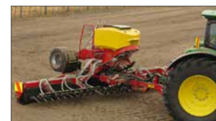
4. Additional seeding equipment for grass sowing or for new grassland.
