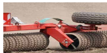
Balanced force transfer to the end section for even soil compaction
