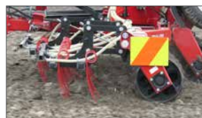
3. Optional Z-roller and 2-rows weeder, or crossboard for cultivation on grasslands.
