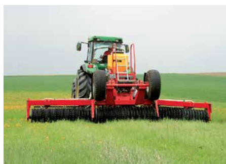
1. Basic frame fitted with the Cambridge roller or smooth roller to suit arable land.
