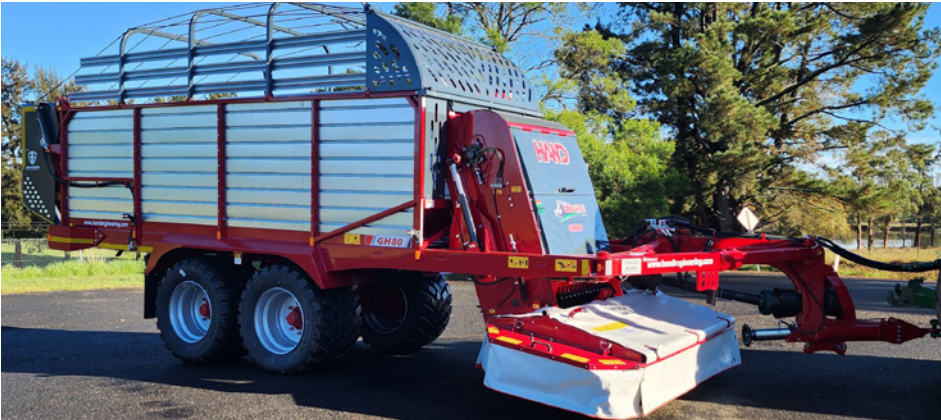
Shotblasted, Two pack primer and paint
